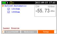
Bidirectional loss test can be performed by just pressing one button to automatically measure and display the entire fiber insertion loss and return loss to help users acquire complete and accurate optical link loss information
