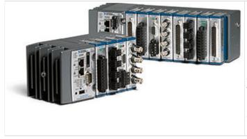
CompactRIO combines an open-embedded architecture with small size, extreme ruggedness, and C Series modules in a platform powered by the NI LabVIEW reconfigurable I/O (RIO) architecture. Each system contains an FPGA for custom timing, triggering, and processing with a wide array of available modular I/O to meet any embedded application requirement.
