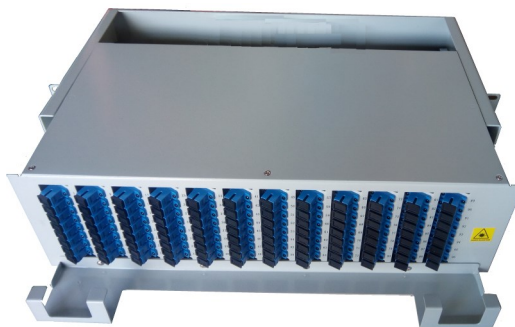
Drawer type, simplex SC, 96 or 120 fiber termination, 3U, with extended table for fiber guides
