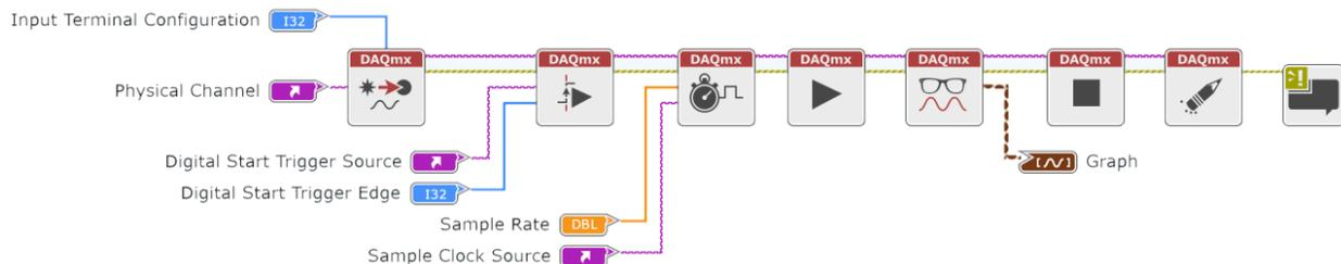
Figure 4. Analog Input Task Designed With the NI-DAQmx Driver and LabVIEW Software
