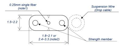
Note 1: Bend insensitive SM fiber must comply with ITU-T.G.652B, G.652D and G.657A. Allowable fiber diameter is 0.25+/-0.015mm.
